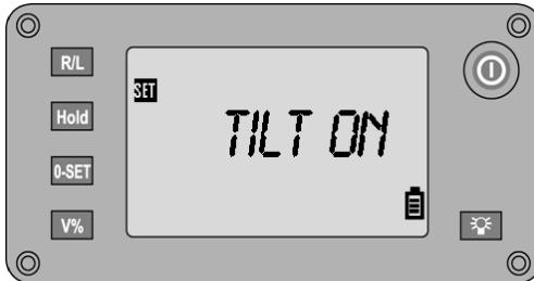
Switching the compensator on / off
