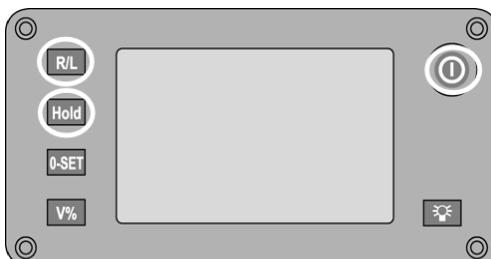
1. Press and hold the **R/L** button and the **Hold** buttons simultaneously and then press the **ON/OFF** button.
