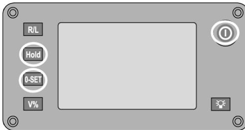
Press and hold the **Hold** button and the **0-Set** button simultaneously.
