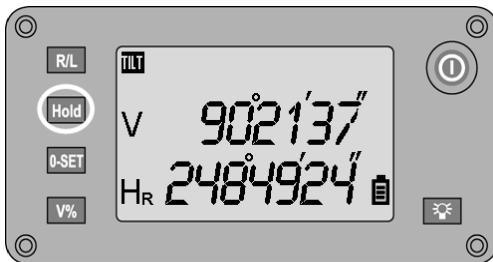
The reading from the horizontal circle can be held by pressing the **HOLD** button, the tool then aimed at the new target and the reading from the horizontal circle released by pressing the button again.
