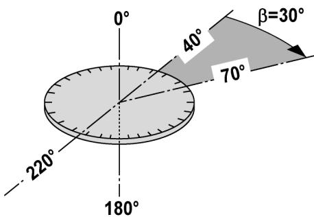
The included angle of  $70^\circ - 40^\circ = 30^\circ$  can be calculated from the horizontal circle readings of  $70^\circ$  to one target and  $40^\circ$  to the other target.
